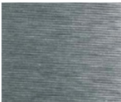
Surface finish: machined, Ra 1.2 μm
